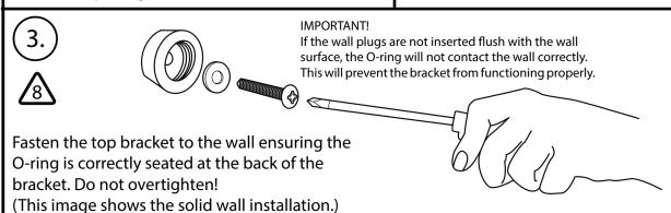
IMPORTANT NOTE: THE TOP BRACKET HAS A SMALLER DIAMETER OUTER FLANGE TO THE BOTTOM BRACKET.
