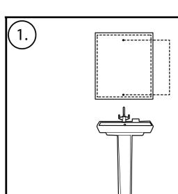
Place the cabinet in the desired position on the wall and mark the position of the top mounting hole. Note that single door cabinets can be positioned with either a left or right opening door. Simply turn the cabinet upside down to change the door opening direction.
