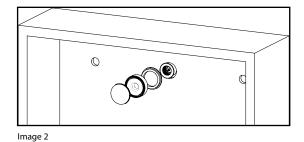
Hang the cabinet onto the top wall bracket, (see image 1) and secure in place by screwing the locking cap and spacer onto the top bracket, (see
