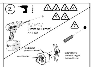
For solid walls drill an 5/16" (8mm) diameter hole in the marked postion and insert a wall plug flush to the surface of the wall. If fitting to a tiled surface, the wall plug should be inserted below the surface of the wall to avoid cracking the tiles.
